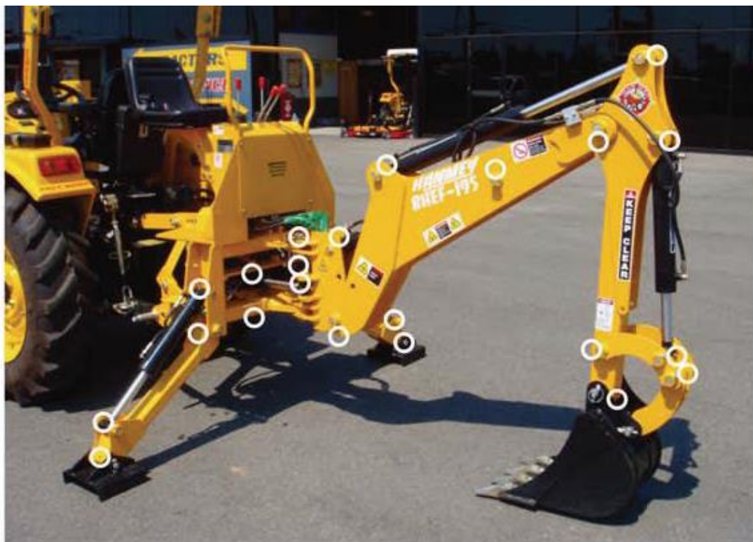
Total of 27 grease nipples on BHEF & BHUF series Grease nipples are located on every moving part
